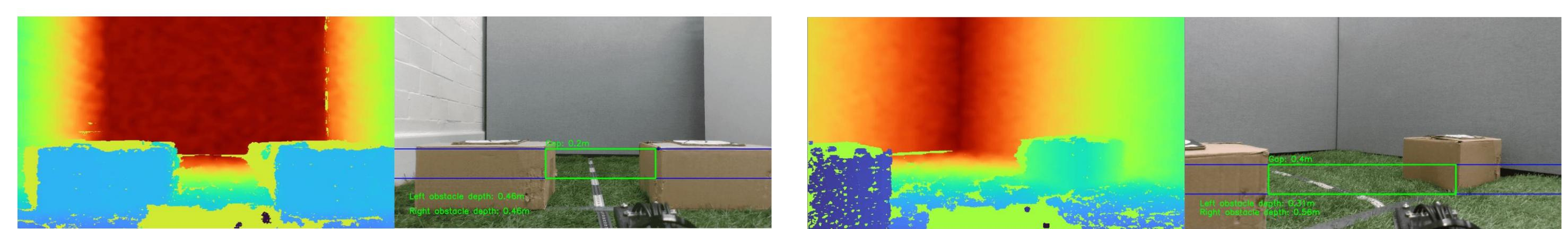
Visual Prediction Algorithm from different approach angles on various obstacles with different apertures. Left: Coloured depth images; Right: corresponding aligned depth-to-colour images with feature info.
