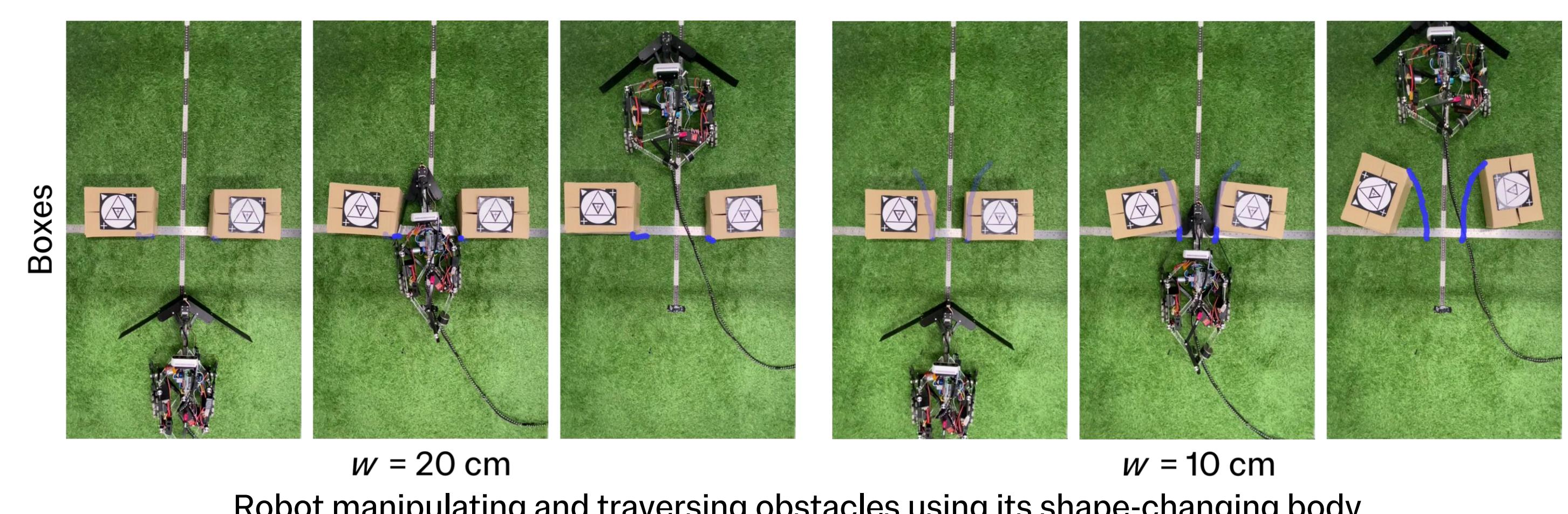
Robot manipulating and traversing obstacles using its shape-changing body.
